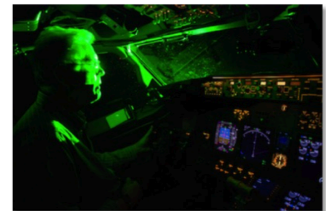
Public domain photo from the U.S. FAA, showing how a laser beam spreads over long distances and can fill the windscreen. The FAA's highest-resolution version is here .
